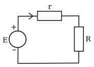
In such a circuit, the electric current *i* is given by  $\frac{E}{r+R}$  and the power *P* delivered to the load *R* is given by  $P = Ri^2$ .
